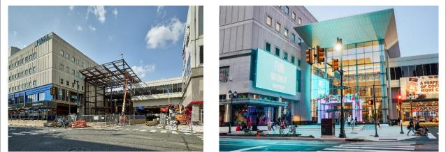
A main goal of the renovation was to create a more open and welcoming destination. The new main entrance, The Cube does so with AESS, structural glass, a column free space with a 68-foot clear span, and clear height of 60 feet.
